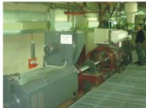
Transient test bed, MAN B&W Holey 5L16/24 engine
