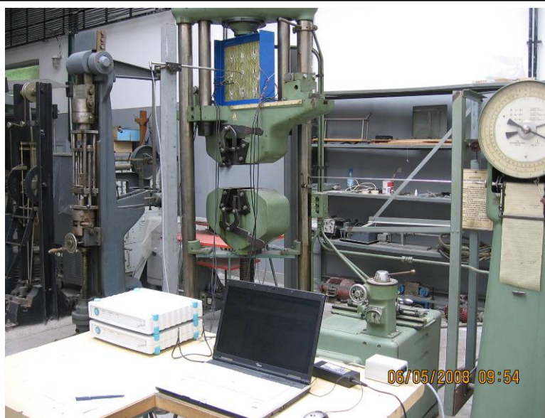
Buckling test on plates made of composite materials
