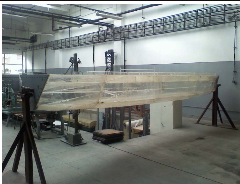
Test on containership structure hull model
